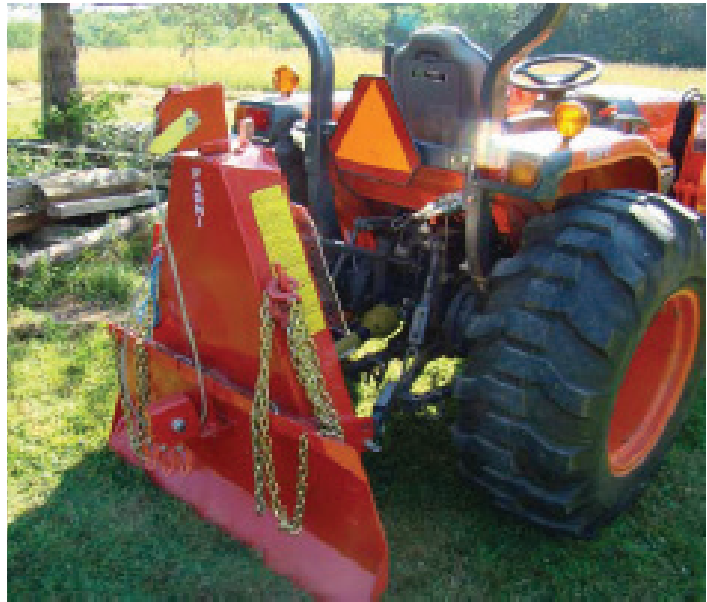
Special attachments for ATV and tractors, shown here with a winch, increase safety and productivity. Care is needed if these types of machines are used for small scale logging.
