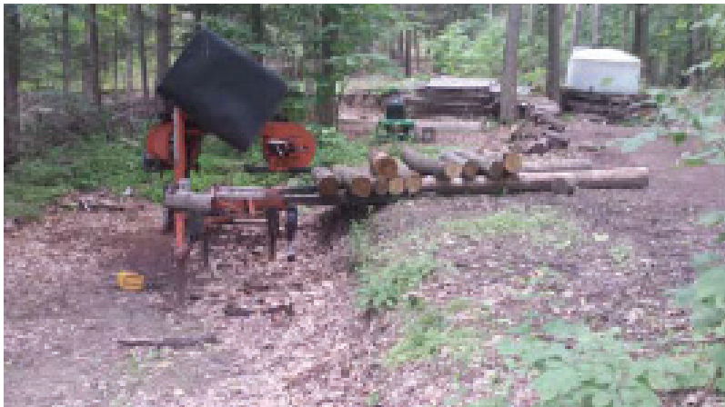
Figure 4. Advance planning will allow arranging logs in a manner to more easily load the sawmill. Creating a cut bank or using a gentle slope makes easy work of loading logs if the sawmill lack hydraulics.
